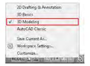
The 3D Modeling workspace is displayed. The Workspaces icon in the status bar indicates that you are now in the 3D Modeling workspace. In this workspace, you can access the various commands and tools needed for creating 3D drawings.
